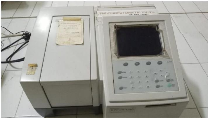
**Gambar 3.4** Alat Spectrophotometer UV VIS
